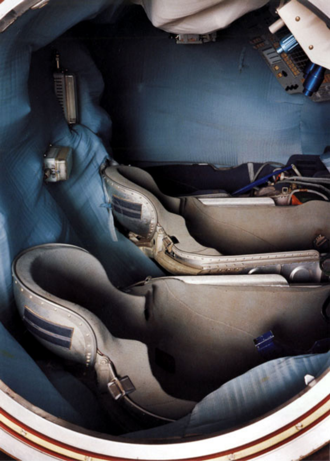
This descent module, with its three cosmonaut couches, is a component of the transport-supply spacecraft developed by Machinostroeniya. The series was designed to ferry crew members and supplies to the Almaz, a large orbital space station intended for military purposes.
