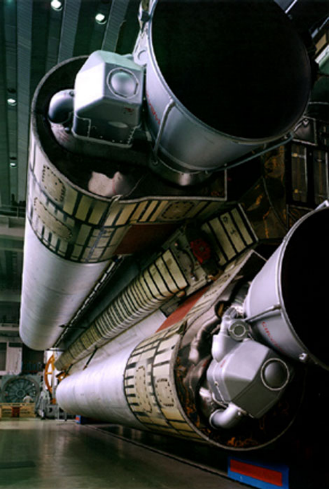
These RD-253-14D14 engines are two of six mounted on the end of a Proton rocket nearing completion at Kurnichev Space Center. The most powerful single-chamber engine produced by Energomash, the RD-253 has been used in the first-stage Proton launch vehicle since 1965 and has operated without a failure since 1969. CREDIT: ADAM BARTOS
